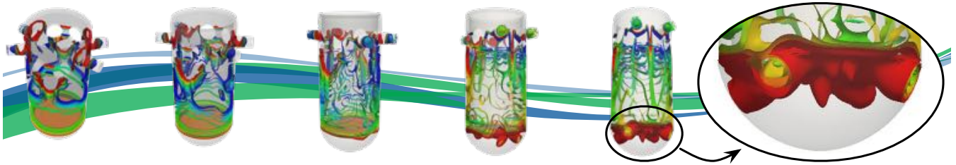
Figure 2: Simulating reactor flow in the lower-plenum during pump startup sequence with Hydra-TH. We see pressure contours in the lower plenum at startup that indicate transient behavior possibly associated with the lower-plenum flow anomaly.
